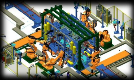
A Tecnomatix simulation of the main geometry station for a new motor vehicle.
