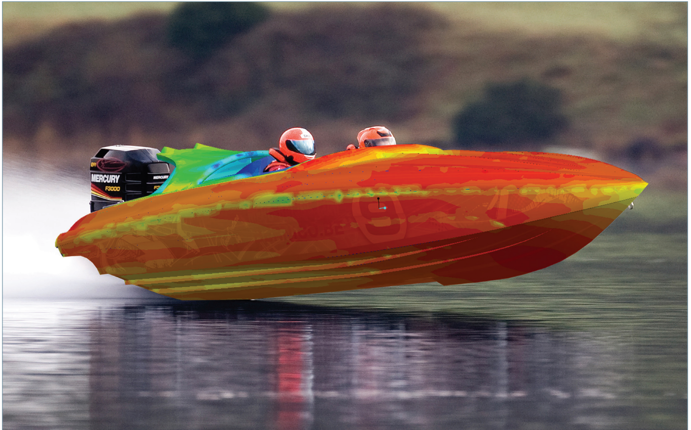
Figure 4: Record-breaking F2 Bernico boat on Coniston Water in November 2009 with superimposed hull pressure contours from Simcenter FLOEFD simulation prediction.
