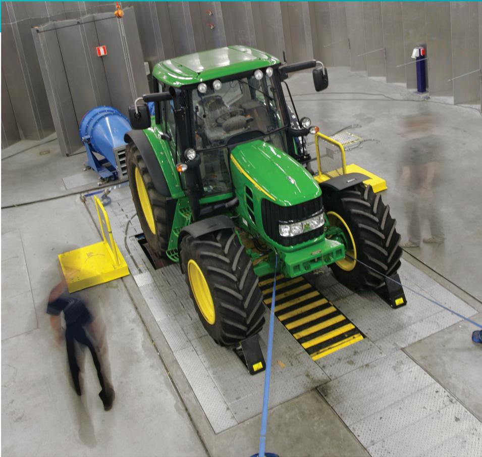
kilometers per hour (km/h) on hard flat road surfaces. John Deere took a number of measurements that showed that a combination of factors amplified the problem, including resonant vibration modes defined by the cab size and shape, cab modal frequencies and associated large sheet-metal parts, and the contribution of different panels to structural sound transmission.
